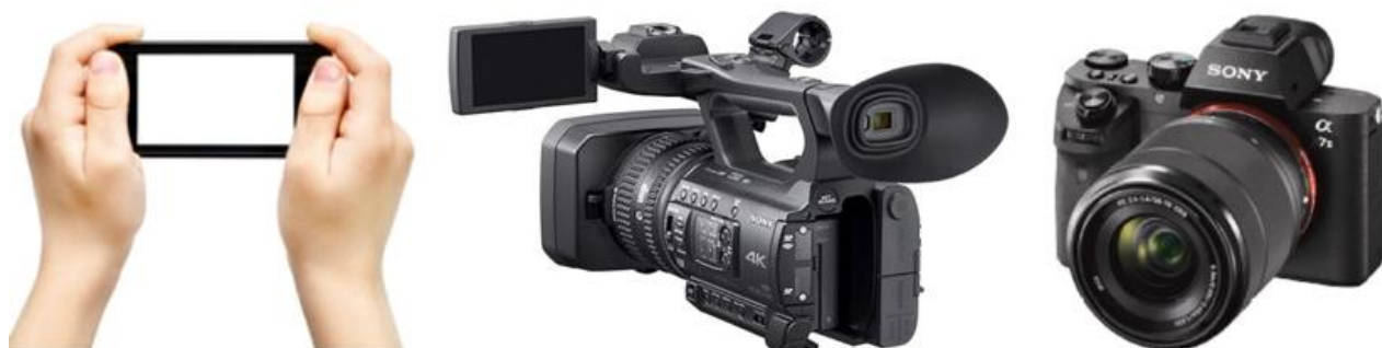
Figure 7. Smartphone, video camera or photo camera: the image quality is good for all of them. The choice of the right device is determined by the application, budget and personal preference. (source: Deliverable 4.3-PLAID)
