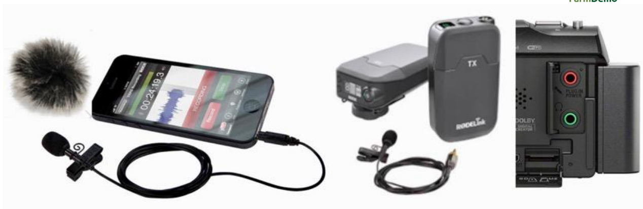
Figure 11. Left: simple microphones with cables for smartphones are already available from €20. Middle: the RodeLink radio link offers a good price-performance ratio. Right: when buying a video camera, make sure that there are connections for microphone (red jack) and headphones (green jack). (source: Deliverable 4.3-PLAID)
